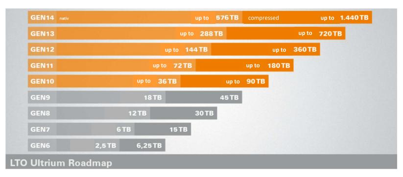
According to a new roadmap, LTO14 should increase the <u>storage capacity</u> of a magnetic tape cartridge to 1,440 terabytes (compressed). This is a factor of 32 compared to the current LTO9 generation, which was released in September 2021 and offers 45 TB of compressed capacity. There is no information yet on the targeted data rates.
